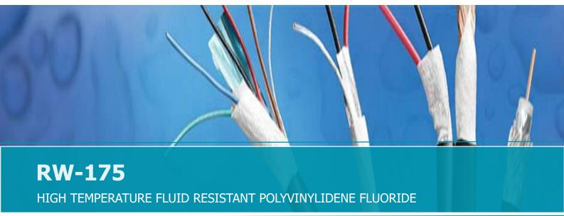
RW-175 is a semi-rigid, polyvinylidene fluoride tubing offering superior cut-through and abrasion resistance. RW-175 is semi-rigid and has excellent resistance to most fuels, solvents and chemicals. RW-175 has a continous operating temperature of 175°C and can easily withstand 300°C for short periods.
