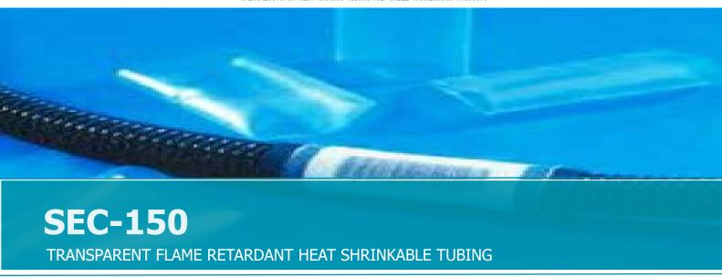
SEC-150 is a 2:1 ratio, thin wall, transparent, flame retardant, heat shrinkable tubing. SEC-150 has been developed primarily for the protection, bundling and jacketing of wires and cables whilst permitting their identification or inspection. It is capable of withstanding extreme abuse, affords UV protection, and operates at high temperatures.
