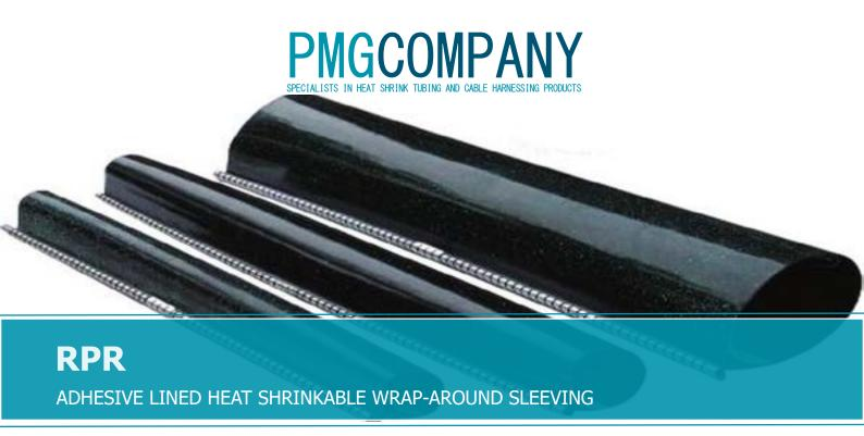
RPR wrap-around sleeve incorporates a stainless-steel channel which is simply slid into position and keeps the wrap-around tubing in place during installation. The wrap-around sleeves are made from thermally stabilised, polymeric halogen free material. The outer surface of the sleeves have thermochromic paint.
