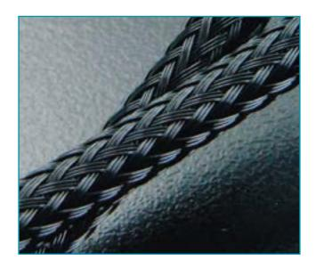
Versaflex serves as an economical means for wire bundling that will trap heat or moisture; expanding easily to fit over irregular shapes then contracting to conform and grip. Hot knife is reccommended for cutting to prevent fraying.
